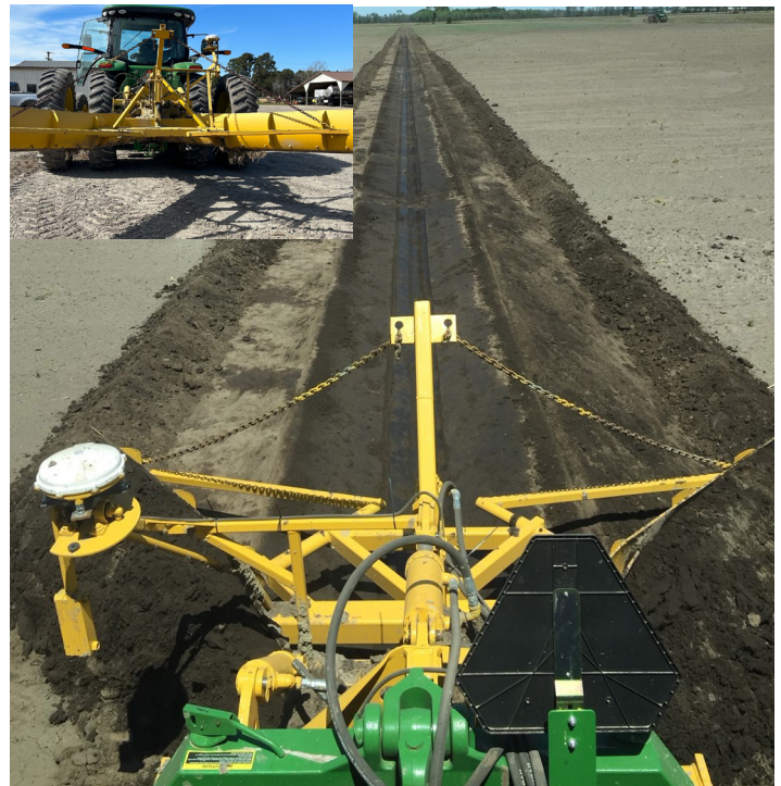
Figure 2- A V-shaped ditcher with GPS grade control to maintain uniform grade (Photo credit: Chad Pool, NC State Univ.).
